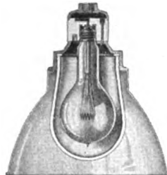
SECTIONAL VIEW OF VAPOR-PROOF FIXTURE WITH BOWL-TYPE REFLECTOR AND PEAR-SHAPE GLOBE
